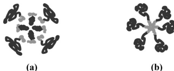
Figure 8. Possible structures for (a) apparently hollow micelles and (b) the spherical micelles observed by TEM.
